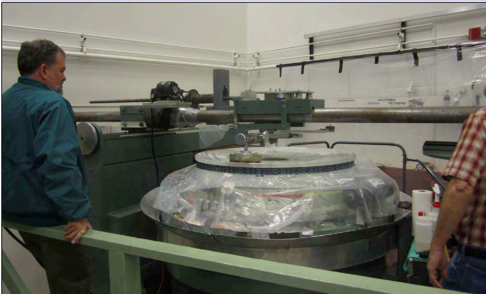
SAO 1.2m primary mirror during a grinding run on December 14, 2011
