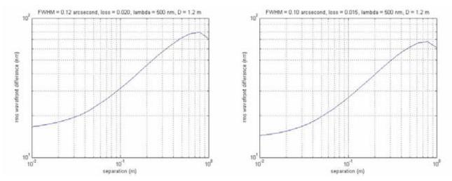
**Figure 1.** Plots of rms wavefront difference (square root of the wavefront structure function) for the specification (left) and goal (right).
