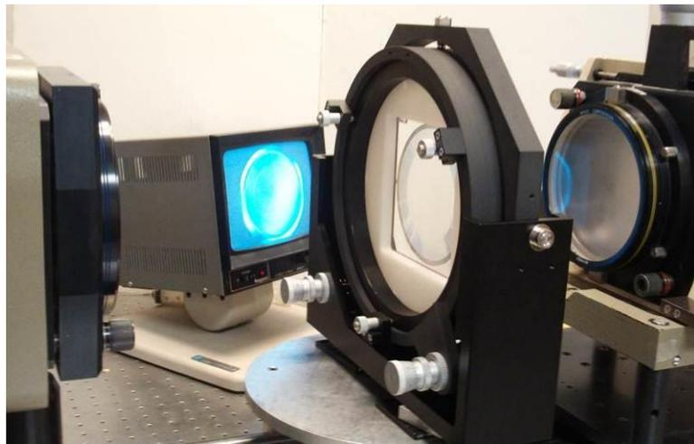
**Figure 4. CGH wavefront error evaluation**
