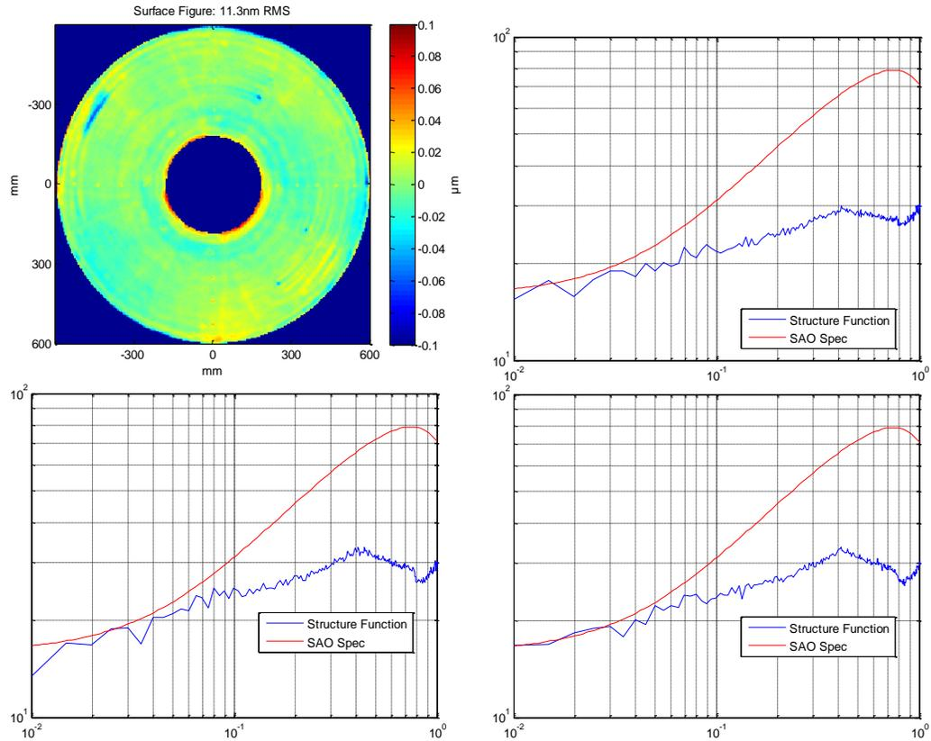
**Figure 13. Structure function analysis of SAO mirror. (Three iterations were conducted to demonstrate repeatability.)**
