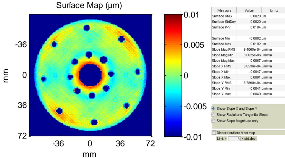
**Figure 7. Residual CGH wavefront error map (Piston, tilt, power and spherical aberration removed)**
