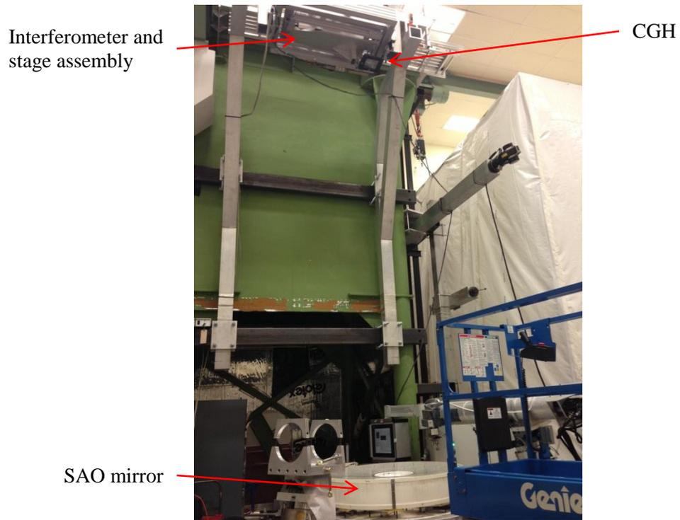
**Figure 3. Interferometric testing set up**
