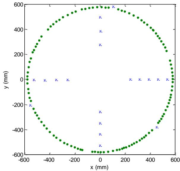
**Figure 9. SAO mirror fiducial layout for distortion correction**
