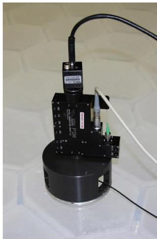
**Figure 14. MFT instrument used for measuring surface microroughness**
