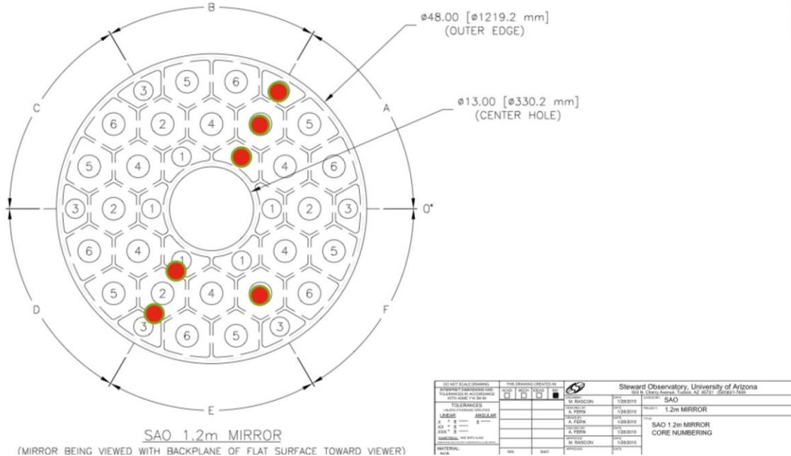
**Figure 15. Microroughness measurement locations on SAO mirror**
