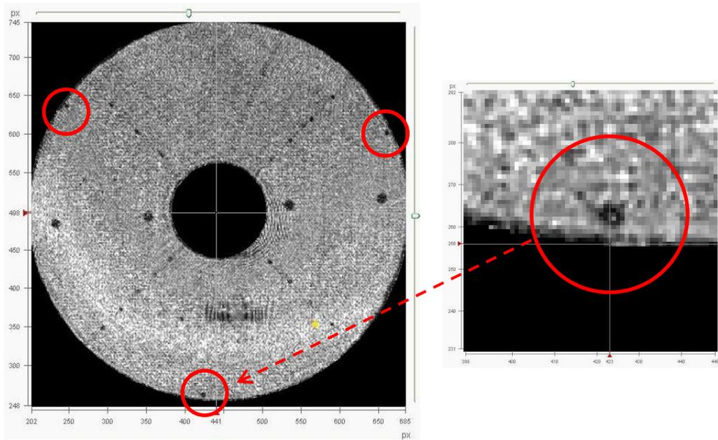
**Figure 10. Modulation map shows three fiducials to verify clear aperture**
