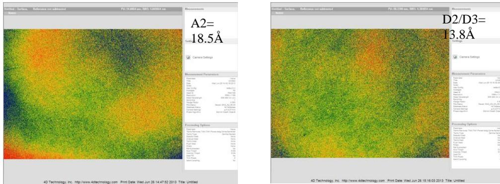
Figure 16. MFT measurements of surface roughness analyzed in 4Sight 2.4
