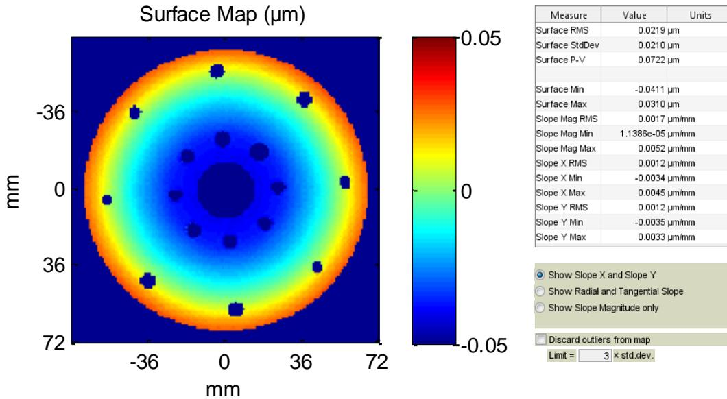
Figure 5. CGH Wavefront error map (Piston and tilt removed and fiducials in CGH are masked)
