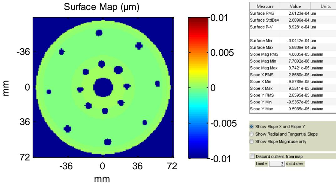
Figure 6. Spherical aberration in CGH
