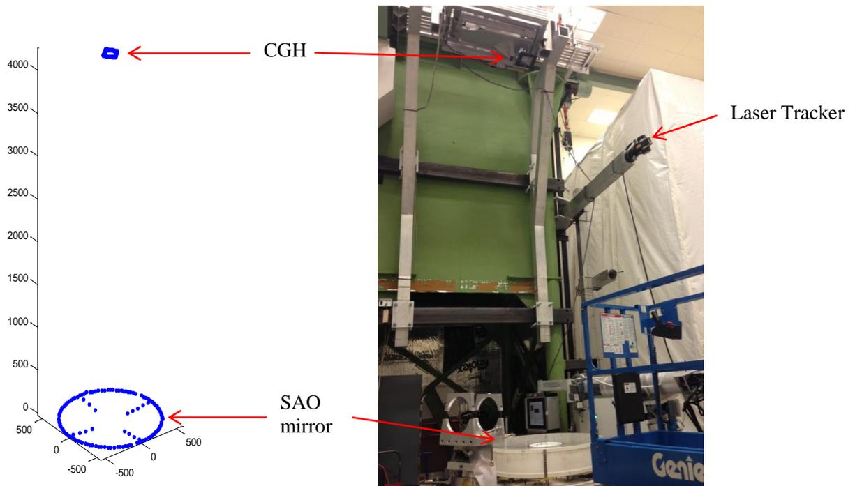
Figure 17. Spacing measurement using a laser tracker
